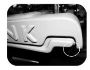
There are four (4) holes under the trim on the front of the unit. The two outer holes move the TRAVEL motor and the two inner holes move the TILLT motor.
