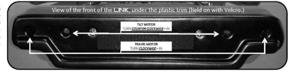
The third motor is the PIVOT and it can be found at the back of the **LINK**. (Shown far right: The backup tool has been designed to curve for the pivot motor, in case your vehicle is equipped with a center console.)
